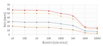
(b) AnchorHash key lookup rate with respect to the number of working buckets for different fixed  $\frac{a}{w}$  ratios. AnchorHash(x) stands for an AnchorHash instance with  $\frac{a}{w}=x$ .
