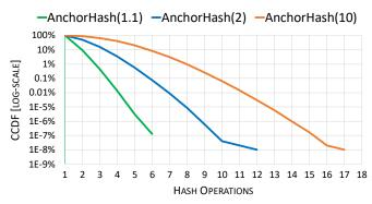
Fig. 6: CCDF for the number of hash operations performed by AnchorHash per key lookup. For example, for AnchorHash(2), 99.9% of keys would require 6 or less hash operations.
