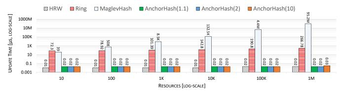
Fig. 8: Comparing update time for resource removals/additions. HRW and AnchorHash require only a few tens of nano-seconds independently of the size of the system. For Ring and especially MaglevHash, the update time increases with the size of the system. For example, for 10<sup>5</sup> resources, MaglevHash requires more than 4 seconds to repopulate its array.
