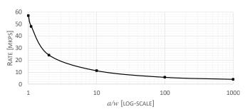
(a) AnchorHash key lookup rate with 1,000 working buckets with respect to different a/w ratios.
