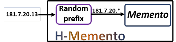
(b) Our HHH algorithm, H-Memento, simply updates Memento with a single random prefix, achieving constant time complexity.
