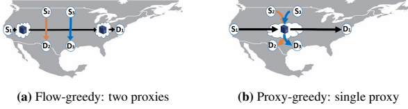
Figure 6: Intuition for algorithm choices. (a) Flow-greedy algorithms pick the best proxy acceleration for the flow that benefits most, even if expensive, and tend to prefer two-proxy acceleration; while (b) proxy-greedy algorithms choose the single proxy that can most benefit the system by serving several flows, thus spending the budget more efficiently.
